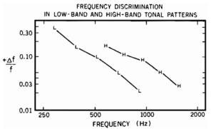
Figure 3. Relative frequency within a pattern is a determinant of frequency discrimination thresholds, in addition to absolute frequency. Average values of delta-f/f for d' = 1.0 are shown for the high- (H) and low-frequency (L) ranges used in Watson *et al.* (1), Experiment 4.Reproduced with permission from (1). Copyright 1975, Acoustical Society of America.
