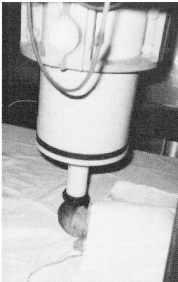
Figure 1. — The SQUID and the neonate during MEG measurement.
