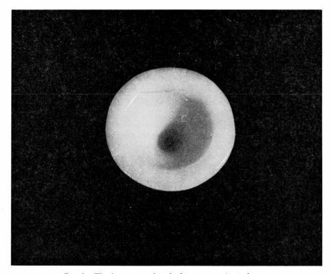
Fig. 2 - The ice cap produced after a two minute freeze.
