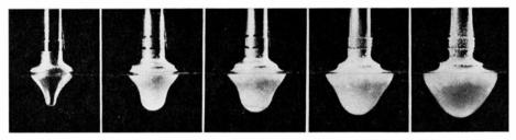
Fig. 1 - A Cryosurgery proble is dipped in an 0.2% suspension of agar. Photographs at 20 second intervals show the build up of freezing. This would be slower in the cervical tissues because of the blood flow warming the area.
