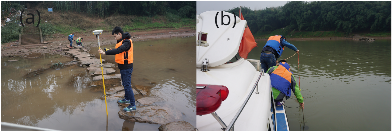
Fig. 3. Field research. (a) Topographic survey. (b) Measuring velocity.
