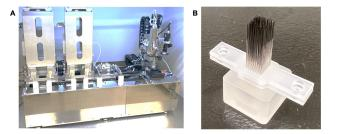
Fig. 2. Bio-3D printer with a needle array (Kenzan). (A) Bio-3D printer. (B) Hollow  $9 \times 9$  needle array (Kenzan).
