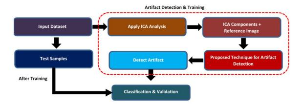
Figure 1. Sparse coding based method proposed for automatic artifact detection and classification of healthy and MDD EEG datasets. ICA is applied to input EEG data which is sent along with the reference image for artifact detection. The proposed technique is applied which detects the artifacts, and finally classification is done to check the validity of the proposed method.
