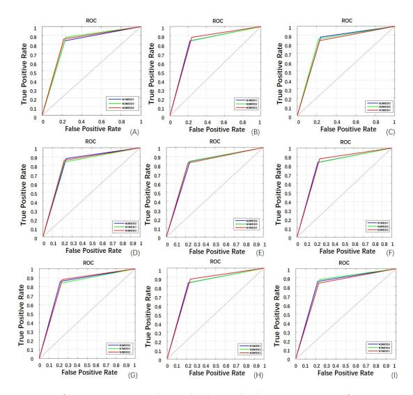
Figure 10. ROC curves for KSVD using SVM, RF, and ELM machine learning algorithms (A, B, C). ROC curves for DTT using SVM, RF and ELM machine learning algorithms (D, E, F). ROC curves for DRT using SVM, RF and ELM machine learning algorithms (G, H, I). The number of 50 iterations were used to determine the ROC using precision and recall metrics. Each ROC shows that N3MMD3 dataset produced better results compared to others.
