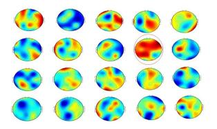
Figure 3. Visualization validation of artifact detection by the proposed model for healthy subject 2 (N2). The artifact detection is done on the  $9^{th}$  channel. The above result uses a minimum distance technique to measure the similarity between reference data and the artefactual component. The detection of the artifact component is indicated with a circle.
