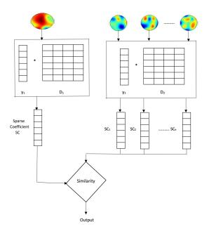
Figure 11. Proposed sparse representation algorithm using dictionary and the minimum distance technique for automatic artifact detection. Sparse coding computes the vector with the smallest number of nonzero coefficients. The primary goal is to obtain the sparse coefficients using the dictionary elements, which is followed by the similarity measured based on the minimum distance approach.
