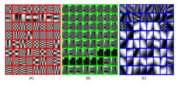
Figure 12. Basis functions used by (a) KSVD, The KSVD-based dictionary elements (or 'atoms') mostly capture singular image points (b) DRT, The dictionary stores image points in well-ordered forms that also capture structural patterns. Moreover, they performed well with smooth and regular patterns. (c) DTT, It also stored image structures well with regular patterns for all dictionary elements using an 8 × 8 EEG signal patch.
