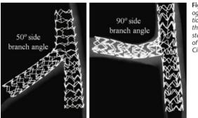
Figure 10. High-intensity Faxitron radiographic images, demonstrating the potential for side branch (SB) ostial coverage of the Xience SBA system. Additional SB stent deployments are shown for SB angles of 50° and 90° (Abbott Vascular, Redwood City, CA).
