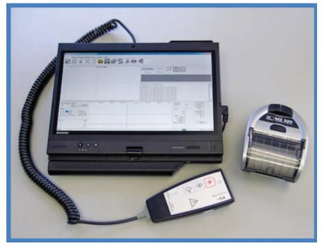
Figure 12. OMNI II programmer for OPTIMIZER<sup>™</sup> IV<sub>2</sub> (Impulse Dynamics Inc., Orangeburg, NY) implantable pulse generators and charger with portable Bluetooth<sup>®</sup> (Kirkland, WA) printer.
