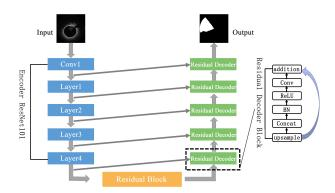
Figure 4. Deep Residual U-Net network structure graph.
