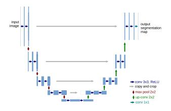
Figure 2. The structure of U-Net segmentation network.
